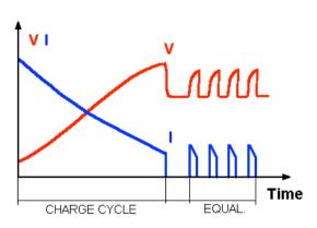
The Charge Controller monitors the entire charging curve, and it incorporates several safety features. The front panel of the MRG charge controller is composed by 4 status LEDs (CHARGING – 80% CHARGED – COMPLETE – FAULT! / ALARM!) and 3 ammeter LEDs.
