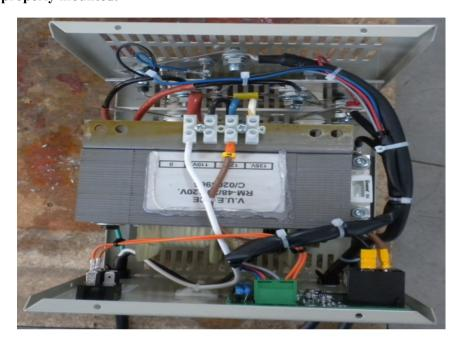
Move the wire to the terminal block correspondent to the measured AC INPUT voltage
