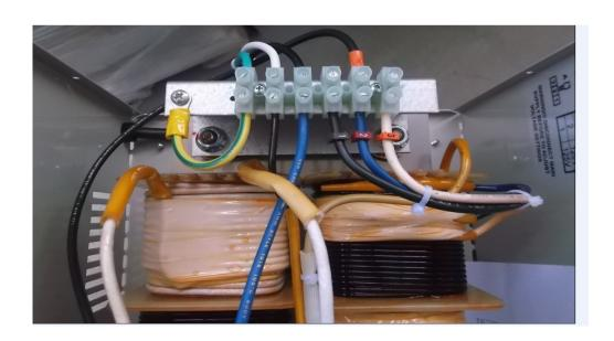
Move the wire to the terminal block correspondent to the measured AC INPUT vol
